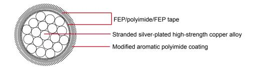
Conductor: Stranded silver-plated high-strength copper alloy conductor
