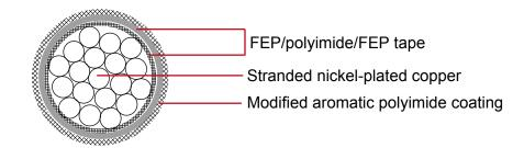
Conductor: Stranded nickel-plated copper conductor
