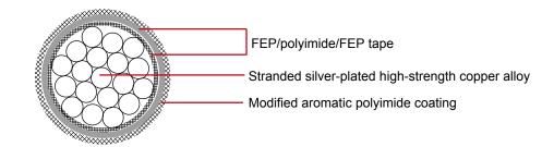
Conductor: Stranded silver-plated high-strength copper alloy conductor
