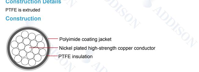
**Conductor:** Nickel plated high-strength copper alloy
