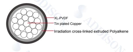
Conductor: Tin plated Copper
